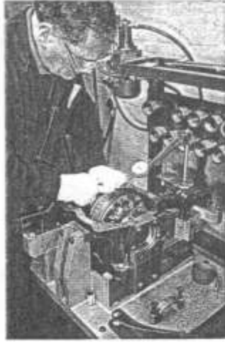
Preloading the bearings
