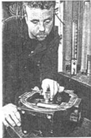
Pinion/diff offset checked
